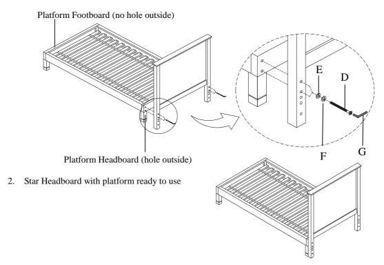
3. Place Star Headboard (A) to the Metal Bed Frame (C), insert spring washer (F), flat washer (E) to the bolt (D). Insert the bolts into Star headboard (A) predrilled hole. Insert flat washer (E), spring washer (F), nut (H) from the back of Scallop onto the bolt (D) and tighten with Allen Key (G) and wrench (I).
