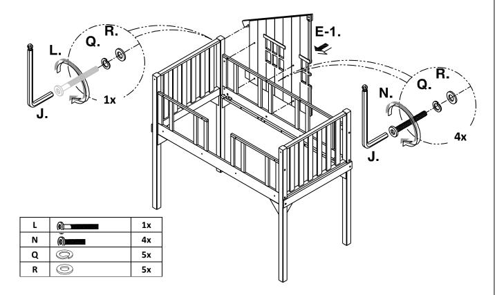
4. Attach the Rear Right Panel (E-2) to Rear Guardrail (C) by inserting (4) Bolts (N) with Spring Washer (Q) and Flat Washer (R) using Allen Key (J). Insert (1) Bolt (L) with Spring Washer (Q) and Flat Washer (R) to secure the Rear Right Panel (E-2) to Headboard post using Allen Key (J). Do not over tighten.
