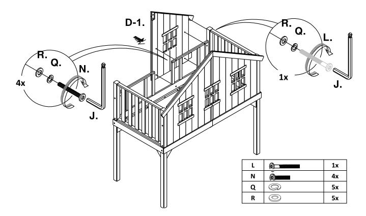
6. Attach Front Right Panel (D-2) to Front Guardrail (B) by inserting (4) Bolts (N) with Spring Washer (Q) and Flat Washer (R) using Allen Key (J). Insert (1) Bolt (L) with Spring Washer (Q) and Flat Washer (R) to secure the Rear Right Panel (E-2) to Headboard post using Allen Key (J). Do not over tighten.
